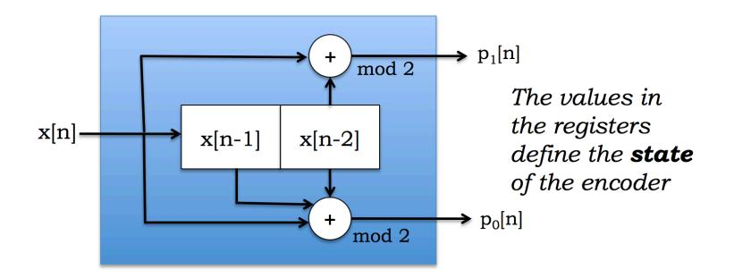
One message bit x[n] in, two parity bits out
